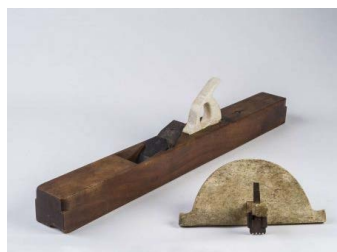
50 SCRIMSHAW WHALEBONE AND MAHOGANY CARPENTER'S PLANE WITH STEEL BLADE, AND A COOPER'S MARKING GAUGE, NINETEENTH CENTURY.
